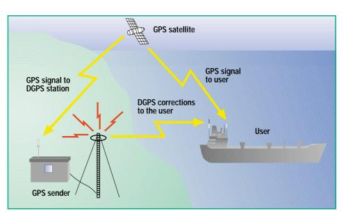
The operating principle of the differential GPS system
